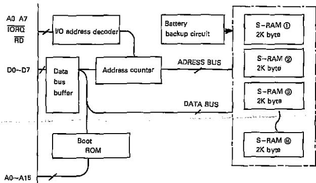
Note The address counter is incremented automatically with the input/output of data.
