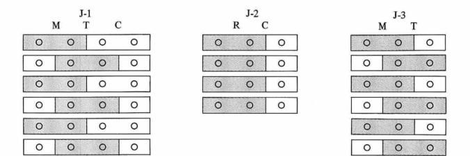
Since port addresses B0H, B1H, B2H, and B3H are used in the program, set the switch SW-1 in the following (factory setting).
