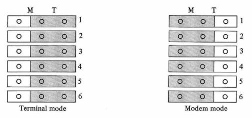
Fig. 4-3 Setting Modes for Channel A (Jumper block J-3)
