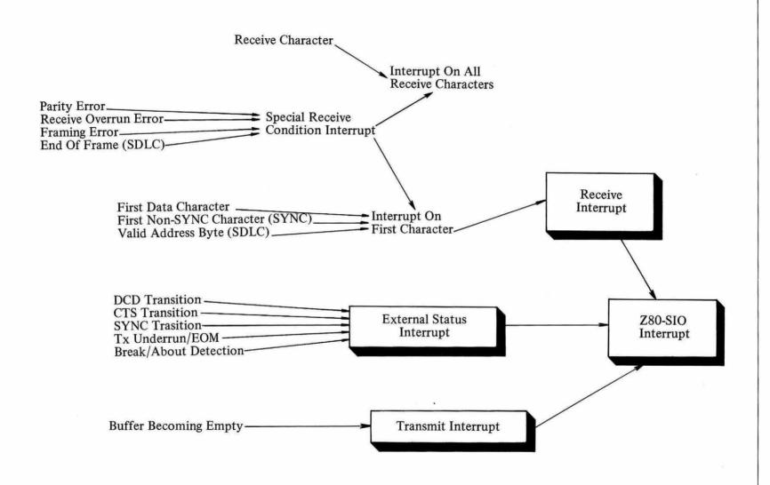
Fig. 6-3 Interrupt Structure
