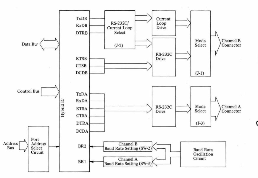
Fig. 10-1 Block Diagram of the Interface Card
