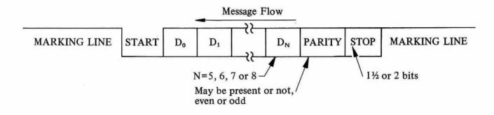
Fig. 6-1 Asynchronous Message Format
