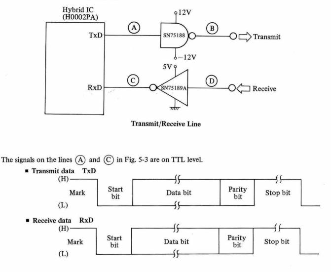
The signals on the lines (B) and (D) in Fig. 5-3 are on RS-232C level.
